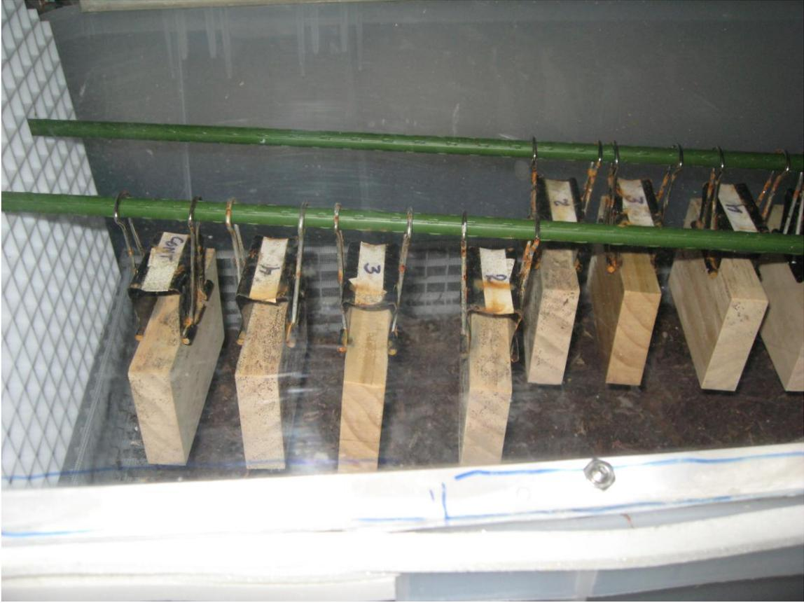
Figure 3. Test and control coupons incubated in environmental chamber
